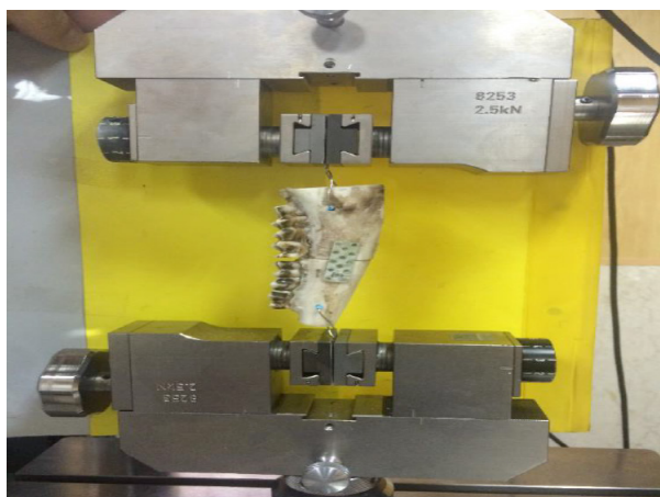
Figure 1. After inserting the bone fragment is fixed with screws and plates on the UTM machine.
