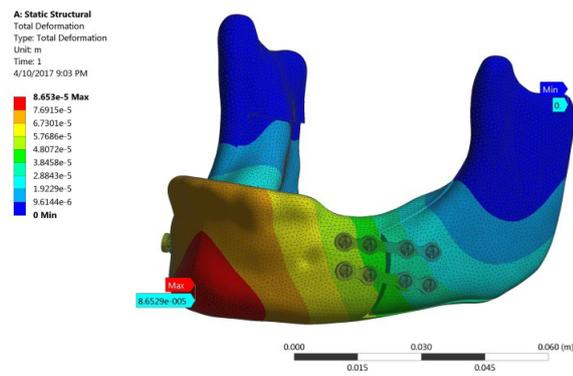
Figure 14. The Two-Parallel Fixation Method, Deformation Contours.
