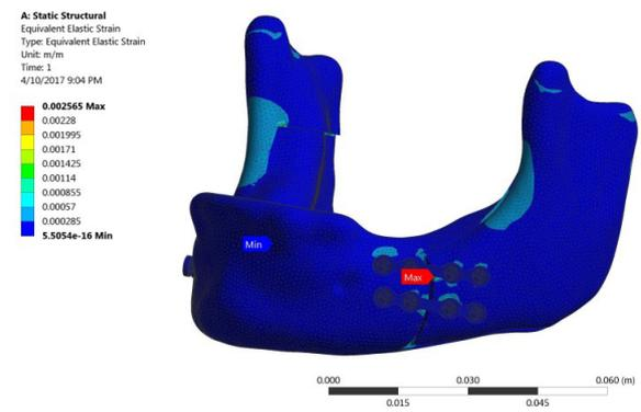
Figure 16. The two-parallel fixation method, strain contours.
