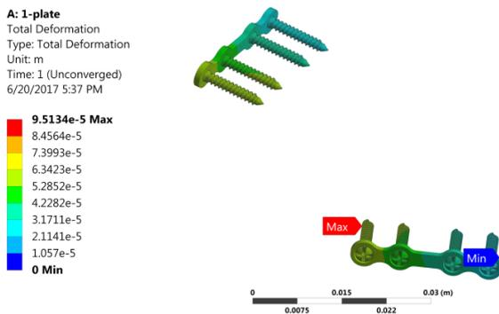
Figure 11. The one-plate fixation method, deformation Contours.
