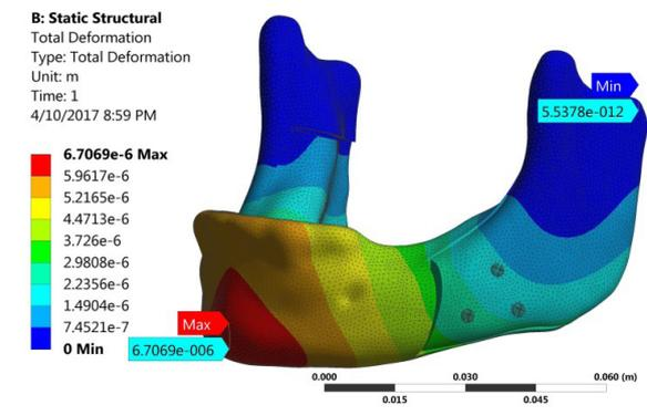
Figure 17. The triangular screw fixation method, deformation contours.
