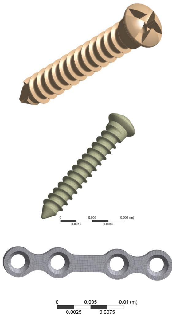
Figure 5. The fixation screw and plate model.
