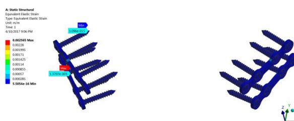
Figure 15. The two-parallel fixation method, stress contours.
