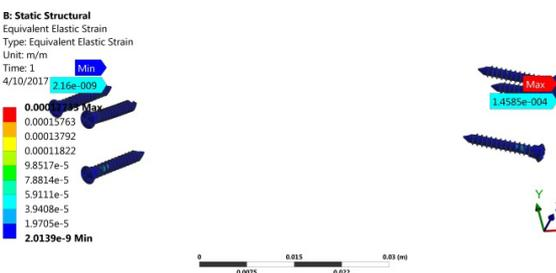
Figure 19. The Triangular Screw fixation Method, Strain Contours.
