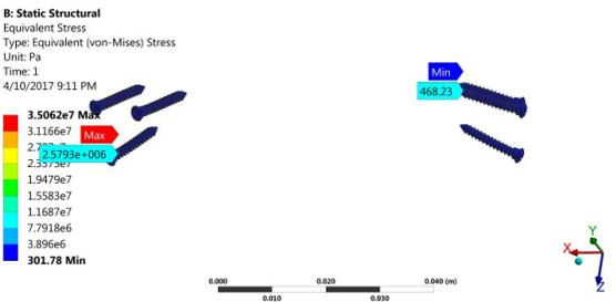
Figure 18. The Triangular Screw fixation Method, Stress Contours.
