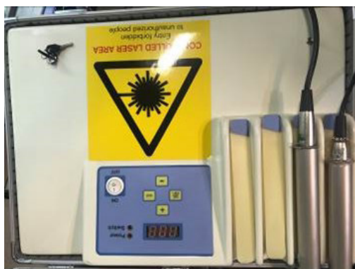
Figure 2. Lasers of blue 485nm (Laser System Ltd, Iran) and green 532nm (Laser System Ltd, Iran) wavelength.
