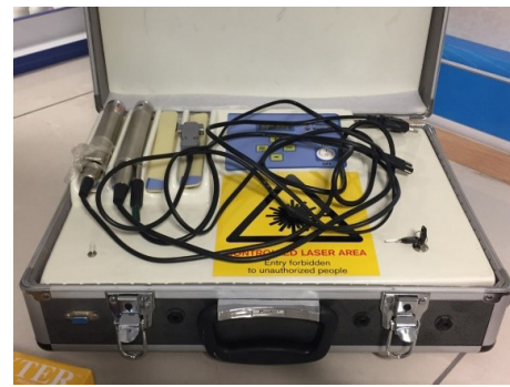
Figure 3. Low-level diode laser (LASER SYSTEM Ltd, Iran) with wavelengths of 485nm, green 532nm.
