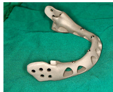
Figure 4. Final fabricated Patient-Specific Implant. The geometrically shaped holes have been removed from the implant to adjust the weight and utilize it as a muscle anchorage.
