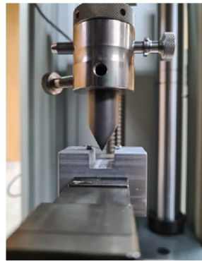
Figure 1. A three-point bending test was conducted using a Zwick/Roell universal testing machine (Zwick GmbH & Co. KG, Ulm, Germany).
