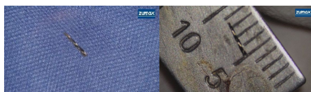
Figure 4. Retrieved fragment measured approximately 3.8 mm in length following removal.
